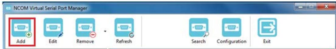
Under “Add connection”, select an available COM port (e.g. COM2. Note that NCOM Virtual Serial Port Manager will show your next available COM port) and type your NCOM device’s IP address and port in “IP Address” and “Remote Port” respectively (e.g. IP Address: 192.168.254.254 Port: 2000). After setting the COM port, IP address and remote port, click “OK” to add a new virtual serial port.
