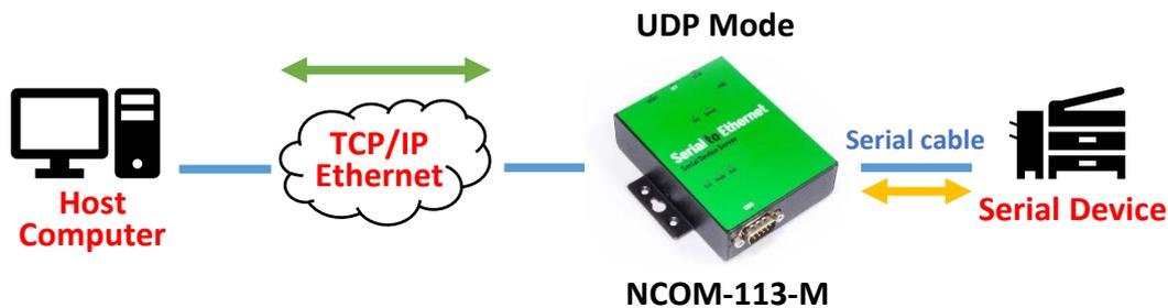
In the figure, UDP mode directly proceeds with data transmission with no connection required.
