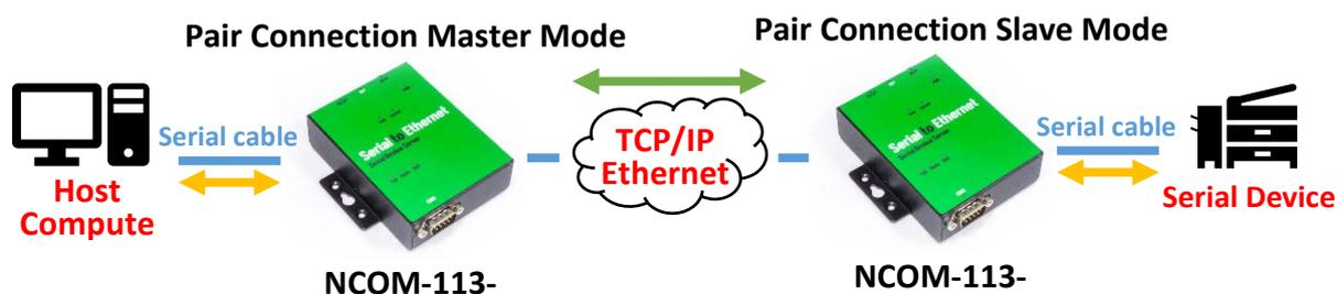
When setting two NCOM-113-M devices in Pair Connection Mode, you need to set the “Destination IP Address” of the master serial device server as the IP address of the slave serial device server.
