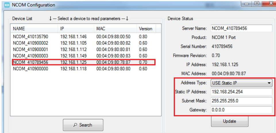
Many networks work in a DHCP network, which assigns IP addresses for client computers and NCOM-113-M automatically. In this case, you need to set NCOM-113-M's IP address to DHCP/AutoIP mode.
