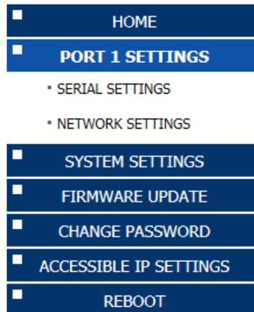
To access the web console interface to configure the device, open any web browser and enter NCOM-113-M’s IP address in the address bar to access the “HOME” page of NCOM-113-M’s firmware.
