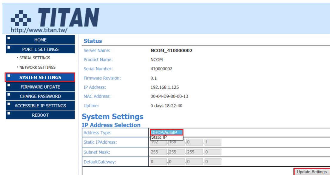
The screenshot displays the NCOM-113-M firmware web interface. The top header features the TITAN logo and the URL <http://www.titan.tw/>. A left-hand navigation menu includes options: HOME, PORT 1 SETTINGS, SERIAL SETTINGS, NETWORK SETTINGS, SYSTEM SETTINGS (highlighted with a red box), FIRMWARE UPDATE, CHANGE PASSWORD, ACCESSIBLE IP SETTINGS, and REBOOT. The main content area is titled "Status" and lists the following information:
