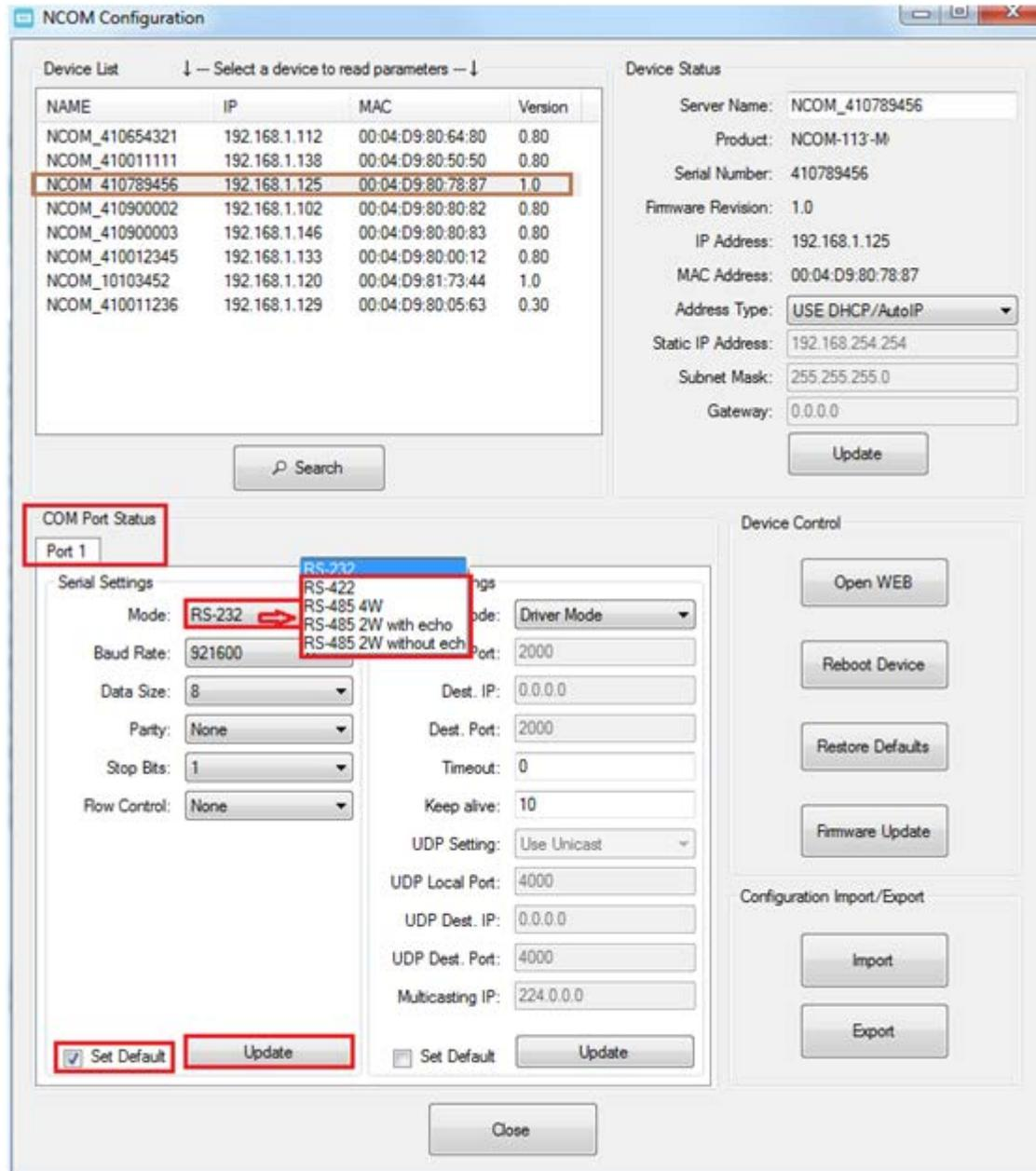
Under the “COM Port Status” window, select “Port 1”. Under “Mode”, select the proper serial port operation mode, then check “Set Default” and click “Update” to set your NCOM-113-M/NCOM-112-M in the proper serial port operation mode.
