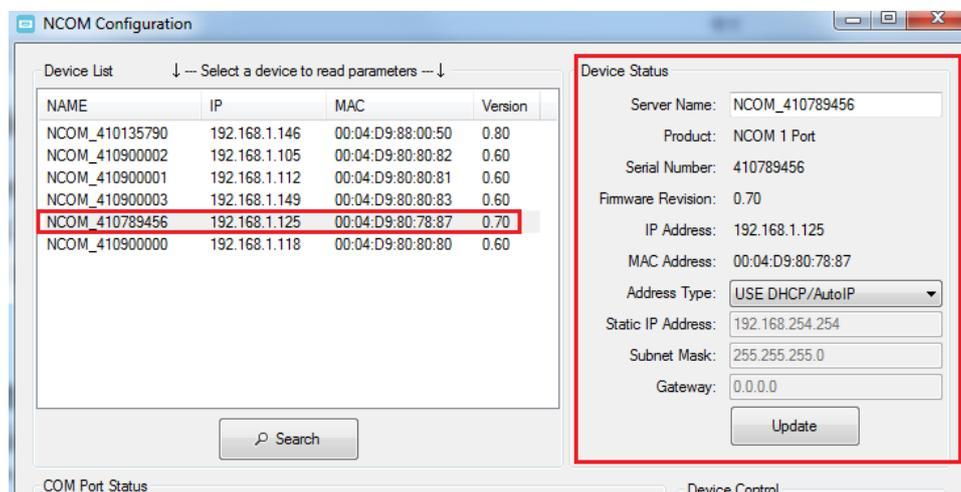
In “Device Status”, you can modify “Server Name”, “Address Type”, “Static IP Address”, “Subnet Mask” and “Gateway” depending on your application.
