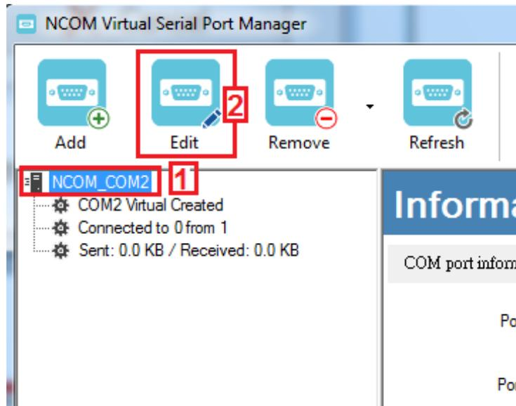
Under “Add connection”, you can change the COM port number with the “COM Port” option (e.g. changing from COM2 to COM3) or change the IP address and remote port with the “IP Address” and “Remote Port” options respectively. After you change the settings, click “OK” to confirm the changes of the virtual serial port for NCOM devices.
