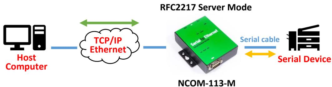
Under the “HOME” page of NCOM-113-M’s firmware, select “NETWORK SETTINGS” to find the “Port 1 Mode Settings” window. Under “Mode”, select “RFC2217-Server” and check the “Make these the default settings” box and click “Apply Changes” to set your NCOM-113-M into RFC2217 Server Mode.
