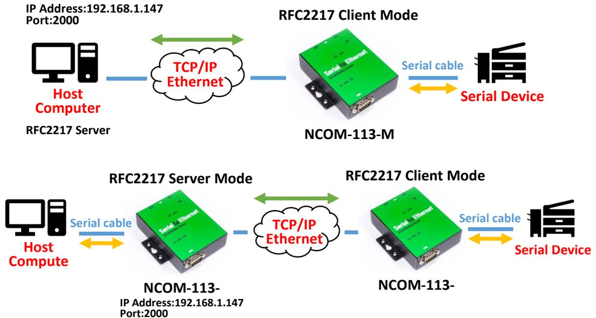
Under the “HOME” page of NCOM-113-M’s firmware, select “NETWORK SETTINGS” to find the “Port 1 Mode Settings” window. Under “Mode”, select “RFC2217-Client” and type “Telnet Server’s IP” and “Port” respectively (e.g. 192.168.1.147 Port: 2000) to establish a TCP connection with a pre-determined host computer or a serial device server. Check the “Make these the default settings” box and click “Apply Changes” to set your NCOM-113-M into RFC2217 Client Mode.
