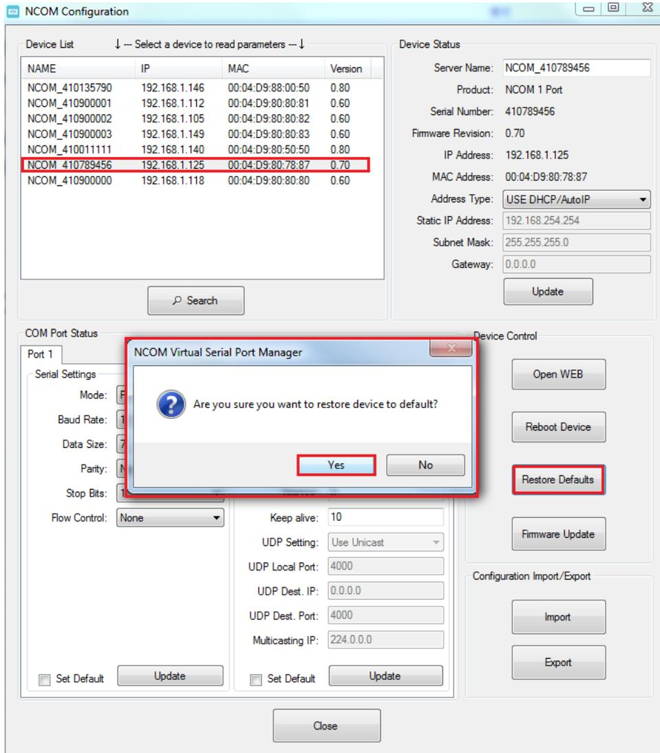
After the NCOM device restores all options to factory default states, a message will indicate “Please refresh device list to read updated parameters!”. Click on “OK” to finish restoring device to factory defaults.
