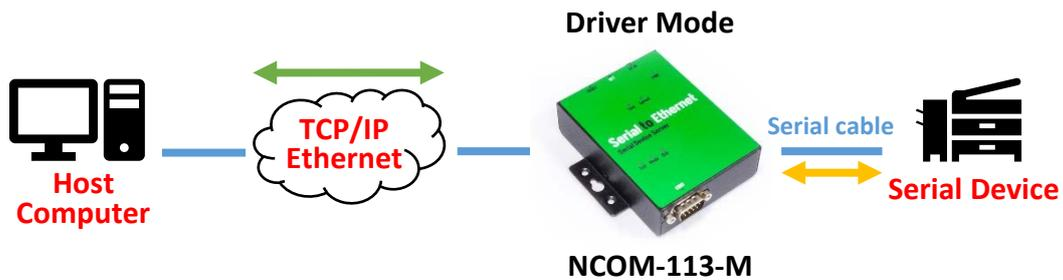
Under the “HOME” page of NCOM-113-M’s firmware, select “NETWORK SETTINGS” to find the “Port 1 Mode Settings” window. Under “Mode”, select “Driver Mode” and check the “Make these the default settings” box and click “Apply Changes” to set your NCOM-113-M into Driver Mode.
