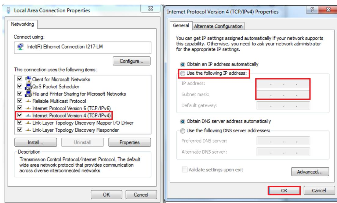
Under “Internet Protocol Version 4 (TCP/IPv4)”, select “Use the following IP address:” and enter the static IP address 192.168.254.XXX (such as 192.168.254.253) and Subnet mask (such as 255.255.255.0) then click “OK” to set your client computer to static IP address.
