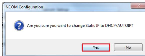
After successfully setting NCOM-113-M to DHCP/AutoIP mode, a message will indicate "Success!!". Click on "OK" to finish changing the IP address type.
