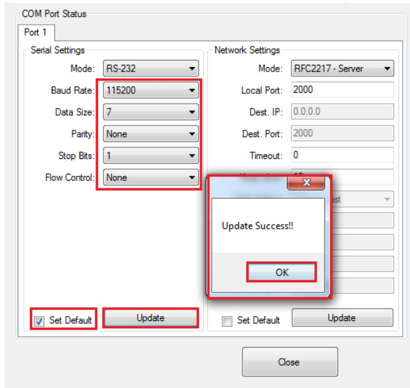
Click on “OK” to finish modifying serial parameters and saving new serial parameters.
