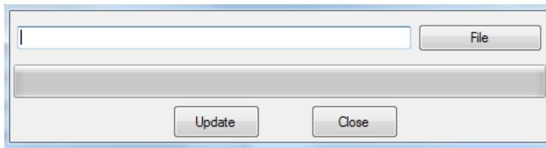
Use the “File” button to browse to the new firmware file and click on “Update” to start upgrading NCOM-113-M’s device firmware.
