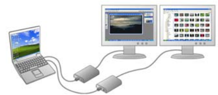
<Extend Mode with 2 Display Adapters>
