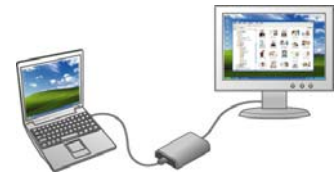
<Extend Mode with 1 Display Adapter>
